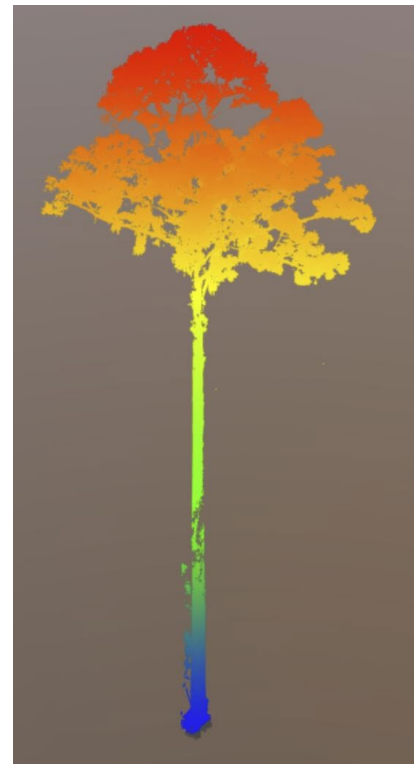
Figure 1. A 3D scan (combined TLS and SfM) of the world's tallest tropical tree.
