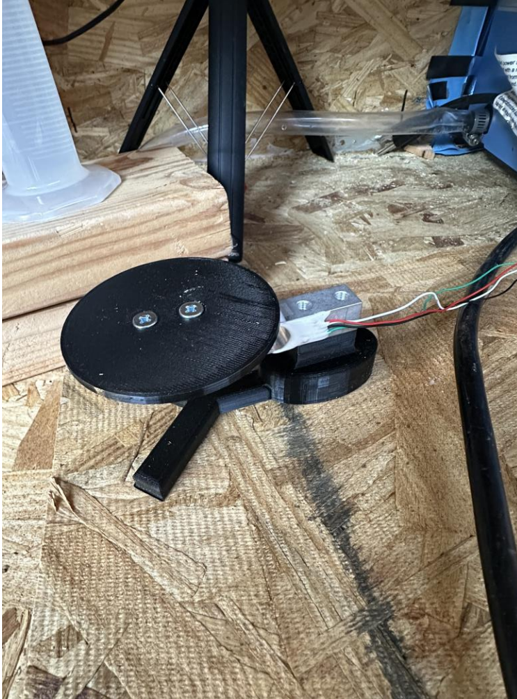
Figure 1: Load Cell with 3D Printed Mount
