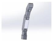
This joint design is a hollow body design for internal tendon routing as well as sensor routing, that features repeating pin hinges and a hinge at the bottom actuates in the opposite direction for the splaying motion. It may be weak to forces due to the hollow body.
