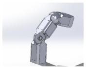
This joint design is two semispherical joint segments that fix together in the middle with a bearing. It offers maximum stability and range of motion. It is not able to easily integrate an angle sensor to the side of the joint.
