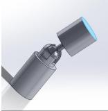
This joint design is a base joint design using a two-way ball and socket joint that is designed for maximum mobility as well as ease of printing. It may have problems with joint angle sensing
