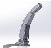
This joint design uses clips to hold each of the joints in place which makes for easy assembly and printing. It also features a two-way ball joint with the clips at the base for the splaying motion. The joints may be weak due to the thinness of the clips.
