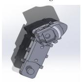
This joint features a slot that allows for an angle sensor and is essential for each joint moving forward. It also has external tendon routing for finger actuation, each of which makes it bulkier but also much more functional
