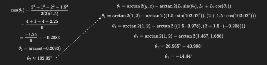
Angles 1 and 2 are found which gives the end of the robotic arm a position of (2,1) with specific arm length values
