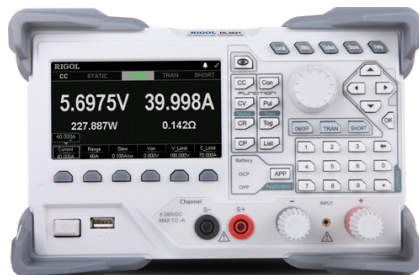
(b) RIGOL DL3201 Programmable DC Electronic Load
