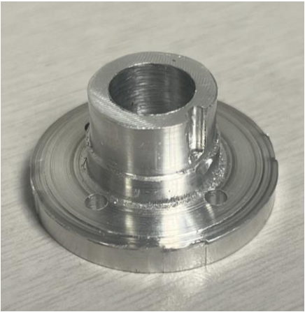
Figure 6: Machined Hub 1st Attempt
