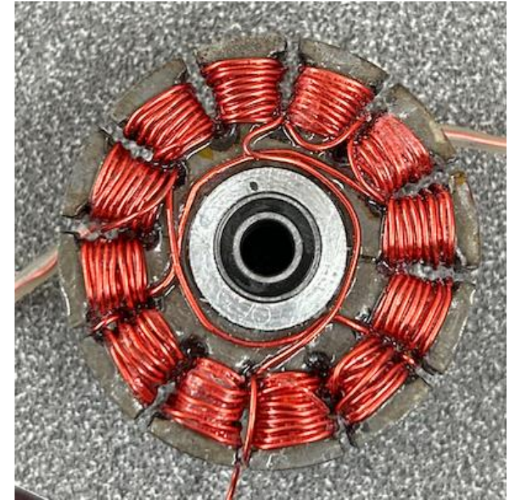
Figure 13: Front Side of Stator
