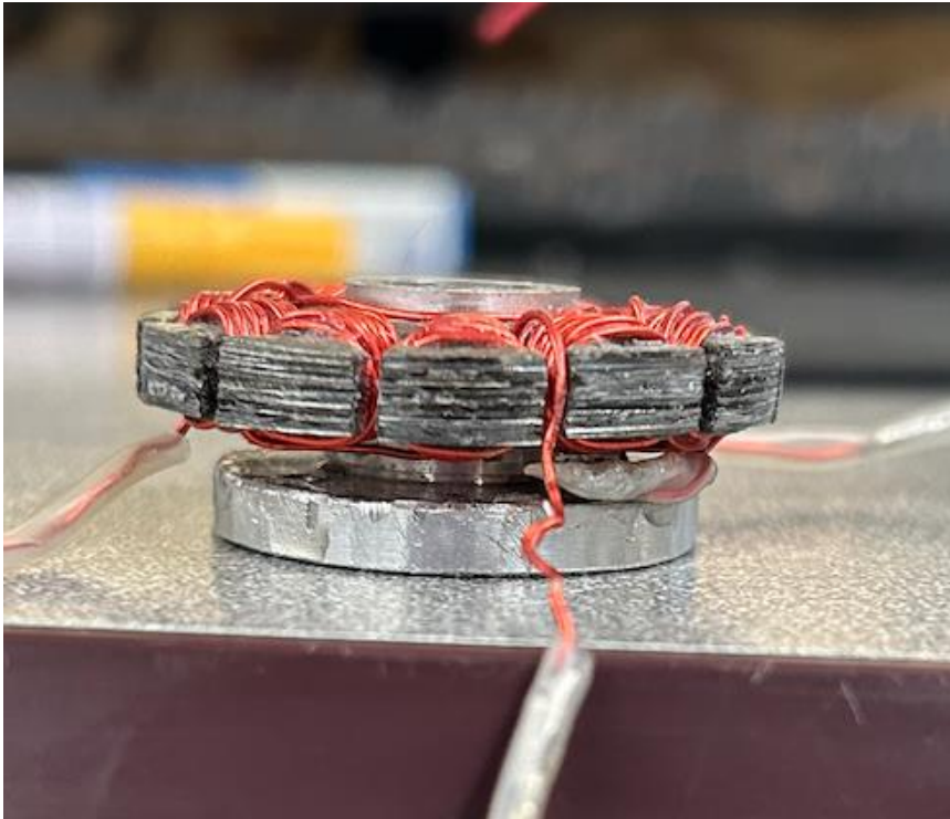
Figure 11: Side View of Stator
