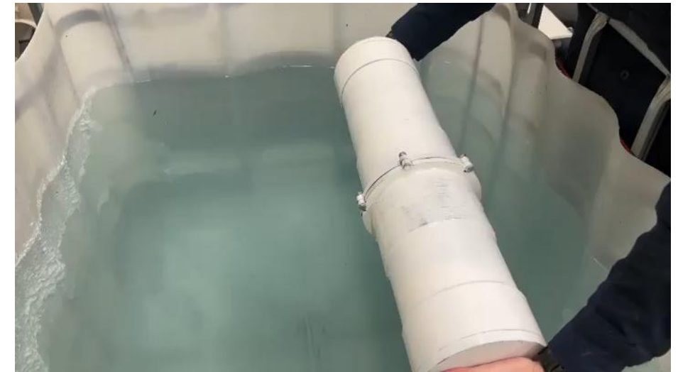
Video [3]: Buoyancy testing in CWC Tank
