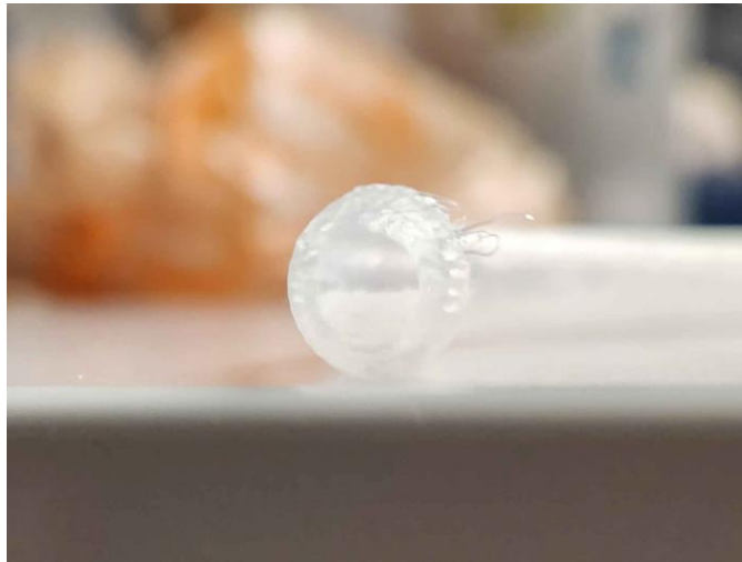
Figure 35 – Lesion Model Adhered to Vessel Model
