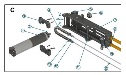
of 89:1 means that the torque output is approximately 3.7 Nm of force
