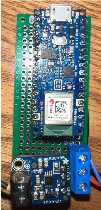
Arduino thermocouple DAQ assembled for testing motor housing thermals
