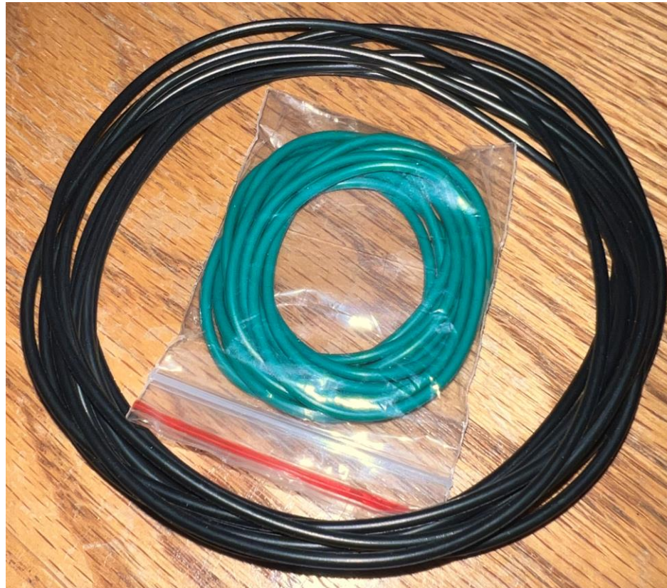
O-rings for motor mount and PCB & battery housing
