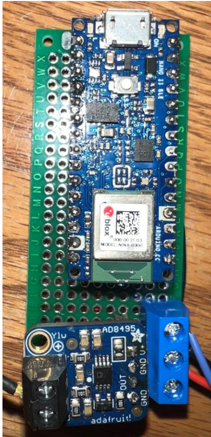
Arduino thermocouple DAQ assembled for testing motor housing thermals
