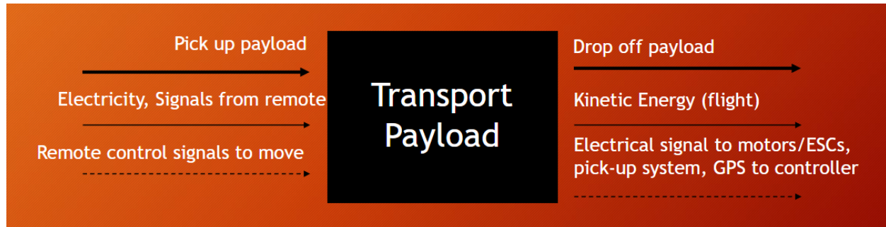
Figure 5.1: Black Box Model outlining inputs and outputs of Drone System
