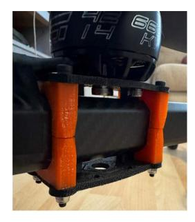
Description: This image showcases how the motors are mounted to the drone's arm(s), the motors are mounted to a mount plate, then connected to the orange arm mounts which clamp around the arm), then a secondary plate is mounted to the bottom, and bolts are routed though the plates and orange the mounts to properly secure the assembly to the carbon fiber arms
