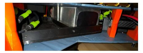
Description: this image showcases how the batteries are secured to their respective bracket using a hold tab that is bolted down in 3 separate mounting locations
