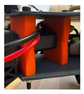
Description: This image showcases how the carbon fiber arms mount to the frame, the orange mounts go around the arm, then bolts are routed through those mounts and are sandwiched in-between the two frame plates, this image also shows how the esc wires are routed in-between the arm and the frame plate in the space between the mounts, and the motor wires are routed through the center of the arms
