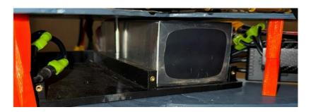
Description: this image showcases how the batteries were mounted to a bracket in the middle section and centered in the body of the drone
