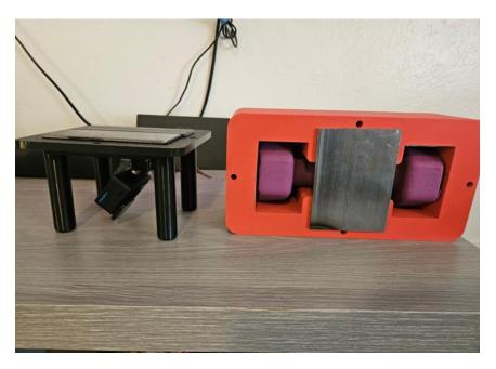
Description: this image showcases the 2 separate payload brackets, the one on the left allows a GoPro camera to be mounted to it in-between its legs, and the bracket on the right allows a dumbbell weight to be mounted inside the bracket, both brackets have metal plates (mild steel) mounted on top of them in order to interface with the magnets from the payload subsystem that is mounted to the drone
