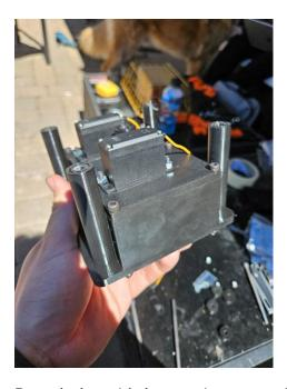
Description: this image showcases how the servos are mounted on top of the magswitches, using a secondary bracket that mounts the servos on top of the magnets
