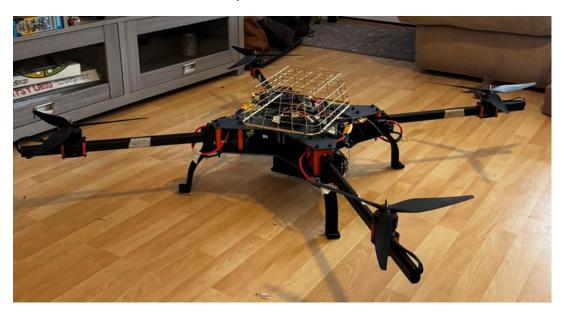
Description: This image showcases the top level, full assembly of the DORIS Drone, in this image the drone is fully assembled, and painted, with all systems fully operational, and electronic system protection (metal basket)
