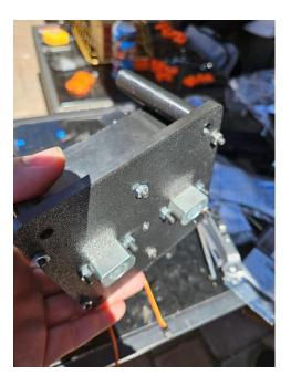
Description: this image showcases how the mechanical magnets (magswitches) are mounted into the payload subsystem bracket, and they are shown protruding from the bottom of the bracket
