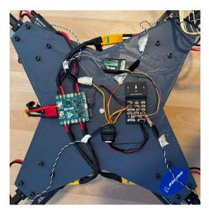
Description: This image showcases how the electronics system was mounted to the top frame plate of the drone, esc power wires and batteries were connected to the power distribution board (PD board), then the esc signal wires, the PD board signal wire, and RC transmitter were connected to the Pixhawk flight controller
