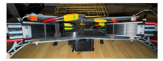
Description: this image showcases how the esc's were mounted in the middle section of the drone body, mounted to the sides of the orange arm mounts (using adhesive Velcro strips); it also shows how the esc's were cross-mounted, each esc for each motor was mounted to the opposite arm, and the wiring is also shown crossed in this image, to be more specific, the esc on the left connects to the motor that is mounted to the arm on the right
