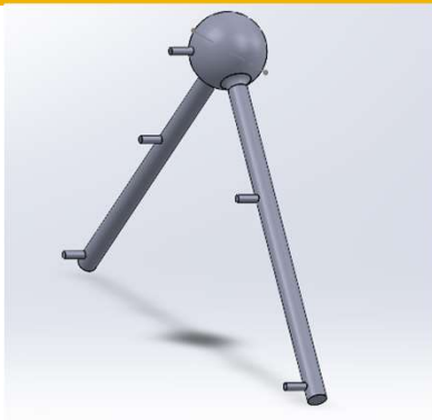
Figure 5: Cylindrical Supports along Structure
