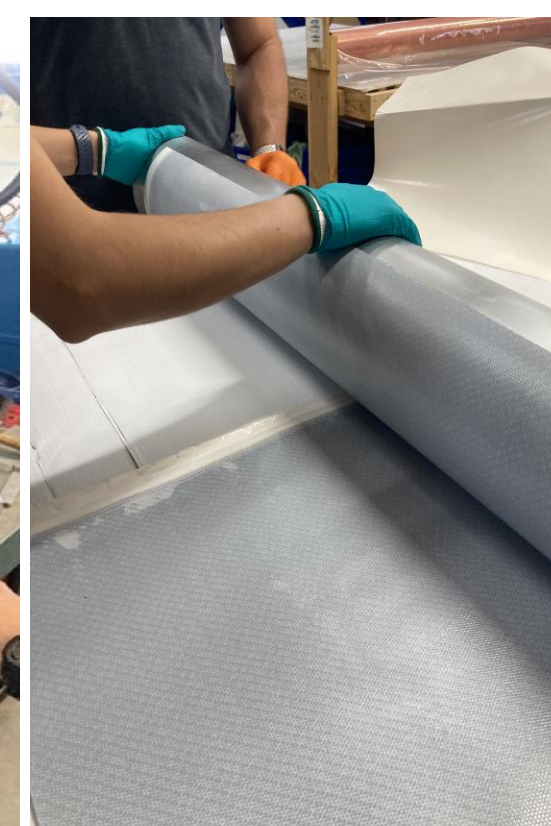
Figure 5: Carbon Fiber lay up (PrePreg)
