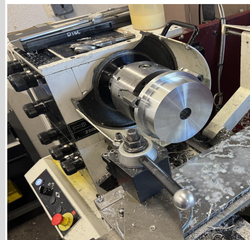
Figure 3: Separation System Part on Harrison Lathe.
