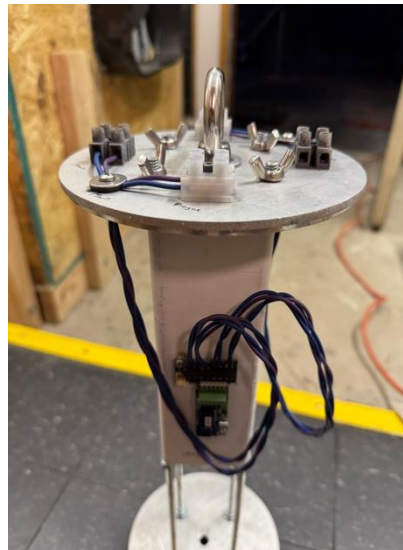
Figure 26: Internal Design of Avionics Bay
