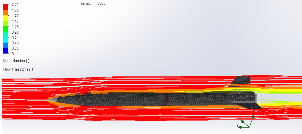
Figure 12: Velocity Flow Simulation of Second Stage
