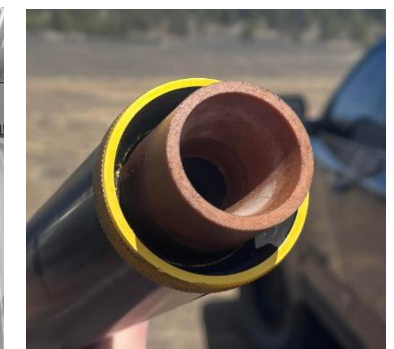
Figure 7. Nozzle Attached to Motor
