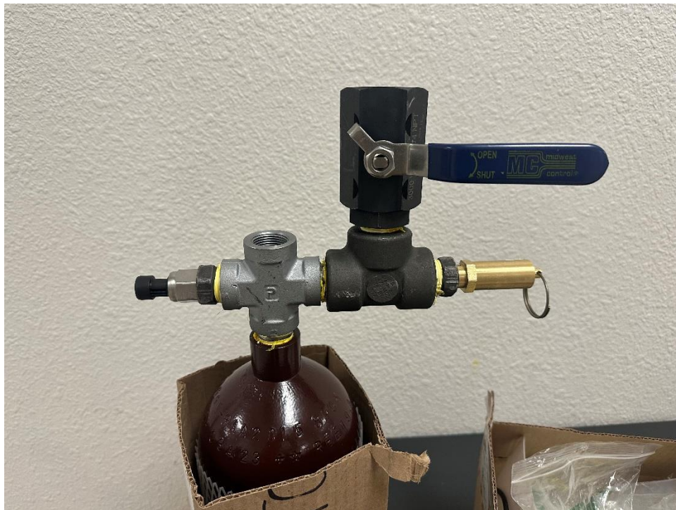
Figure 2. Completed View of Strand Burner
