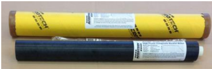
Figure 7. Aerotech High-Power L875DM-PS 75 mm Motor [6]
