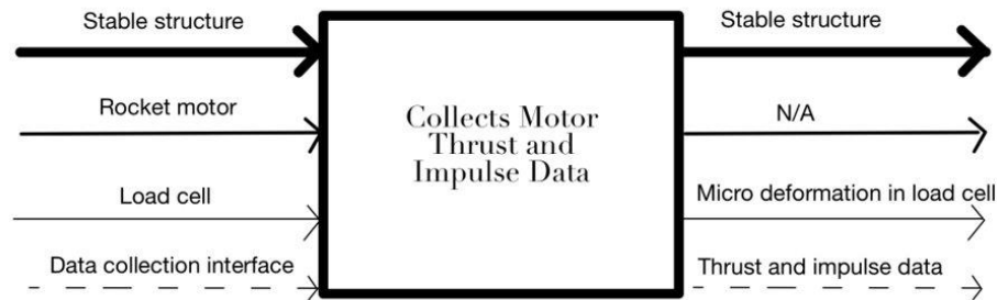
Figure 16. Black Box Model for Test Stand
