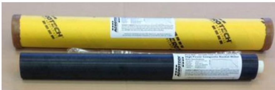
Figure 7. Aerotech High-Power L875DM-PS 75 mm Motor [6]
