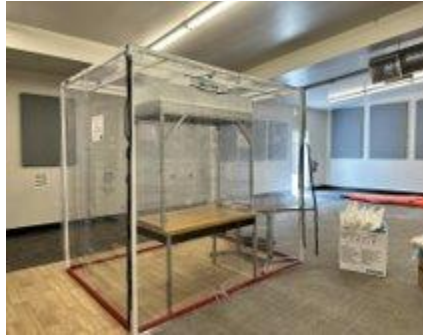
Figure 1: Current Cleanroom Design
