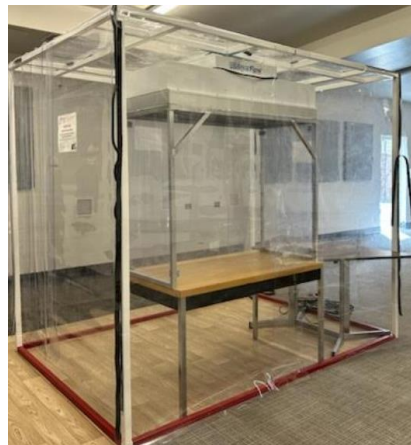
Figure 11: Current Cleanroom Design
