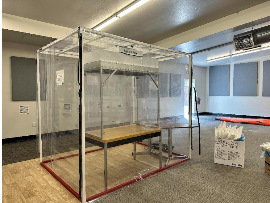
Figure 2: Fume hood and current cleanroom to be converted to gowning room [6]
