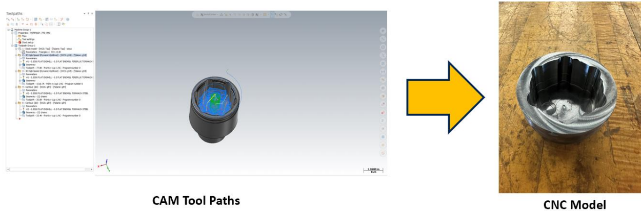
Figure 110: CV Cup Machined Prototype
