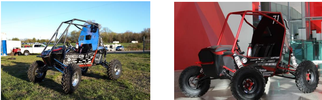
Figure 12: Front (left) vs Rear (right) Frame Bracing
