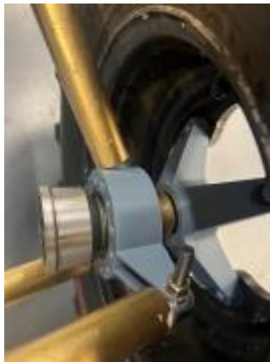
Figure 106: Issue where the holes on hub do not line up to wheel holes. Also, the camber link's rod end is were too big for the knuckle.
