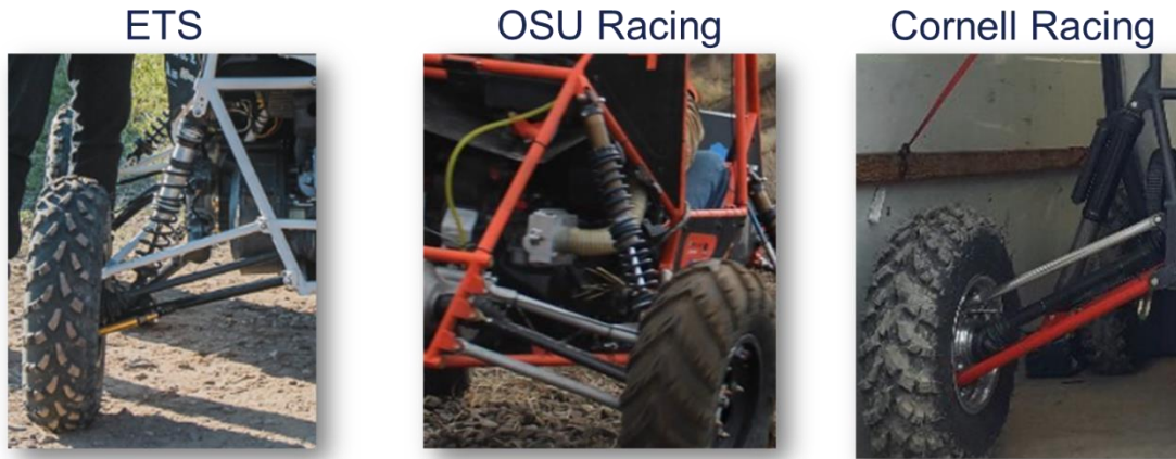
Figure 9: Examples of Rear Double A-Arm Suspension Systems
