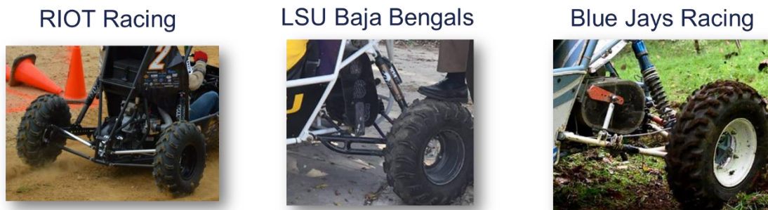
Figure 8: Examples of Rear Trailing Link Suspension Systems
