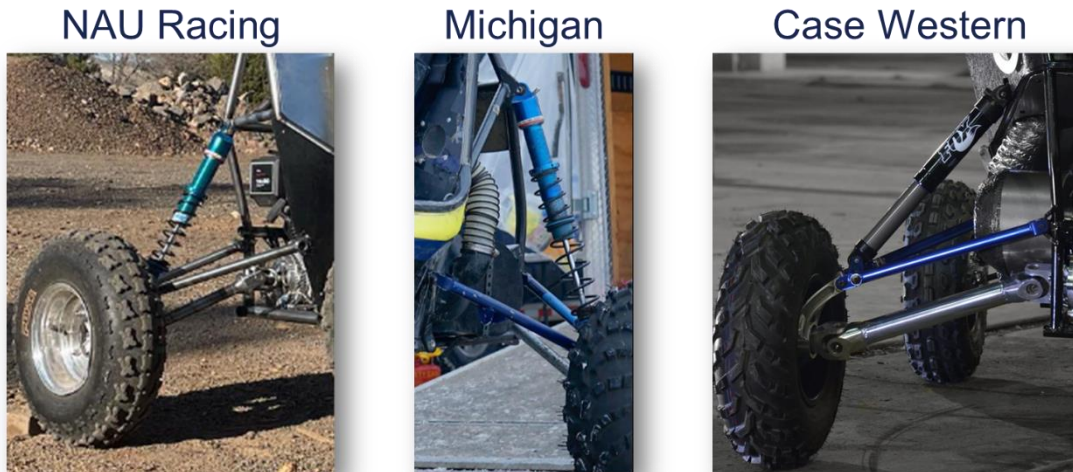
Figure 10: Examples of Rear Single H-Arm Suspension System
