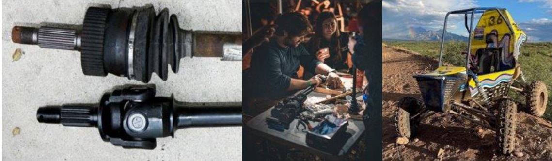
Figure 11: CV Joint and U Joint Comparison
