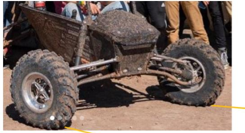
Figure 7 : Cornell's use of Ackermann Steering
