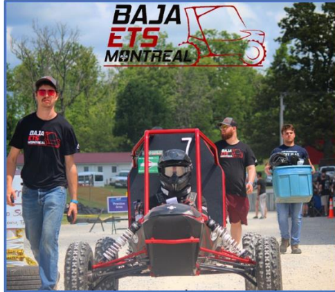
Figure 5: 2023 ETS SAE Baja Vehicle Utilizing a Lower Front Brace and Upper Control Arm Mount
