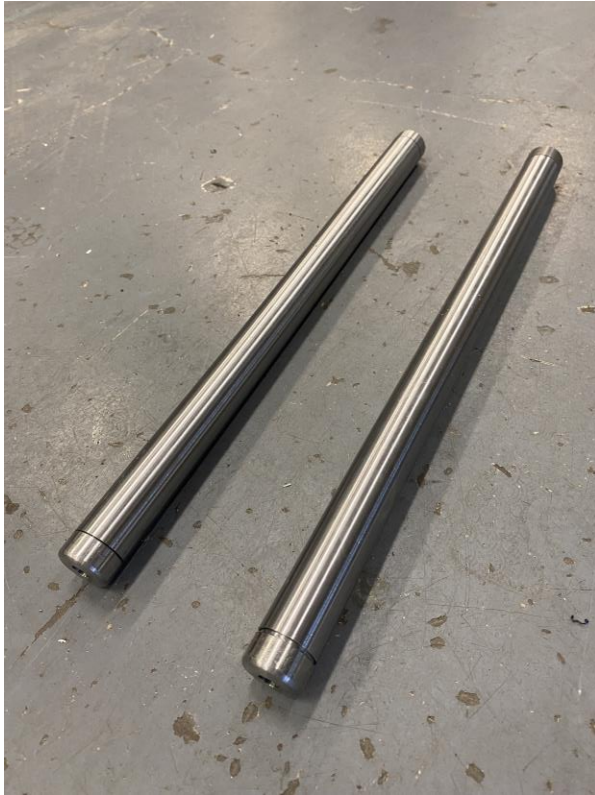
Weld Inserts to tubing
