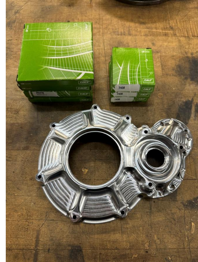
Manufactured Drivetrain Components: Left (Right-Rear Gearbox Intermediate Shaft), Center (4340 Stock for Front and Rear Gears), Right Image (Rear Gearbox Passenger Casing and Bearings & Seals)
