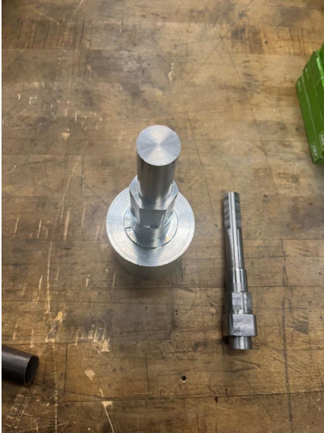
Manufactured Drivetrain Components: Left (Right-Rear Gearbox Intermediate Shaft), Center (4340 Stock for Front and Rear Gears), Right Image (Rear Gearbox Passenger Casing and Bearings & Seals)
