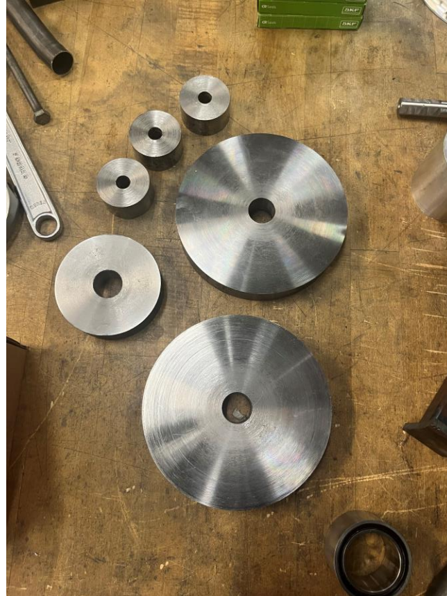
Manufactured Drivetrain Components: Left (Right-Rear Gearbox Intermediate Shaft), Center (4340 Stock for Front and Rear Gears), Right Image (Rear Gearbox Passenger Casing and Bearings & Seals)
