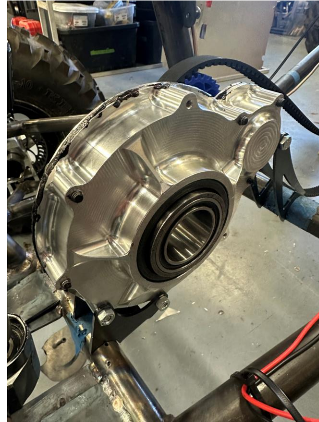
Front & Rear Gearbox and eCVT Assembled in Vehicle, Dog Clutch Housing Bolted on to Rear Gearbox
