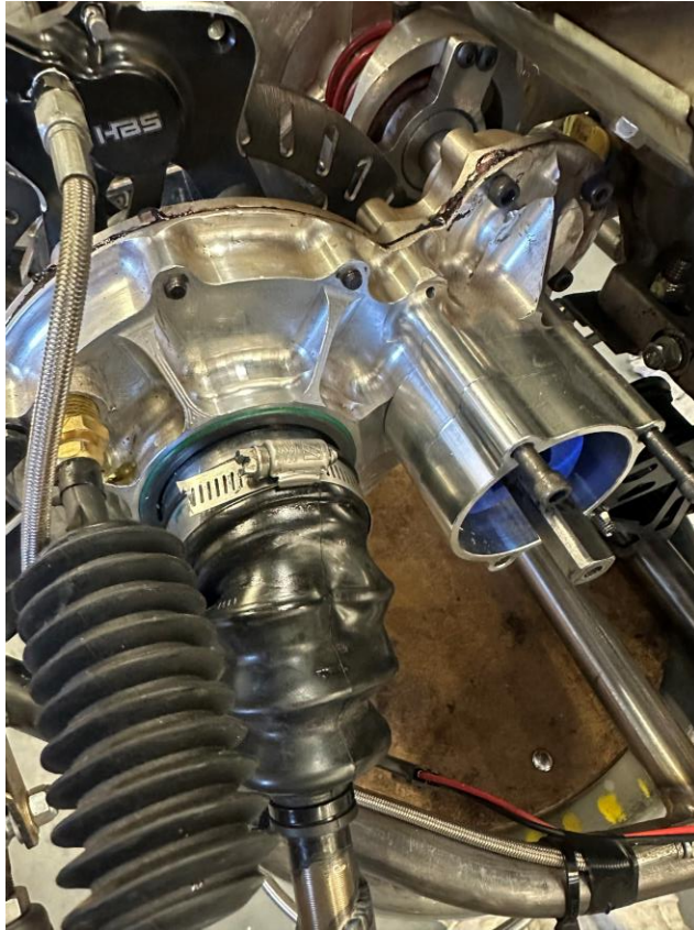
Front & Rear Gearbox and eCVT Assembled in Vehicle, Dog Clutch Housing Bolted on to Rear Gearbox
