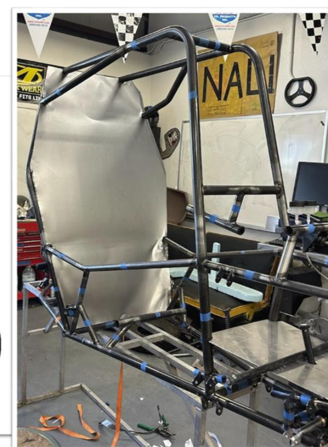
Figure 4: Roll Cage With Firewall
