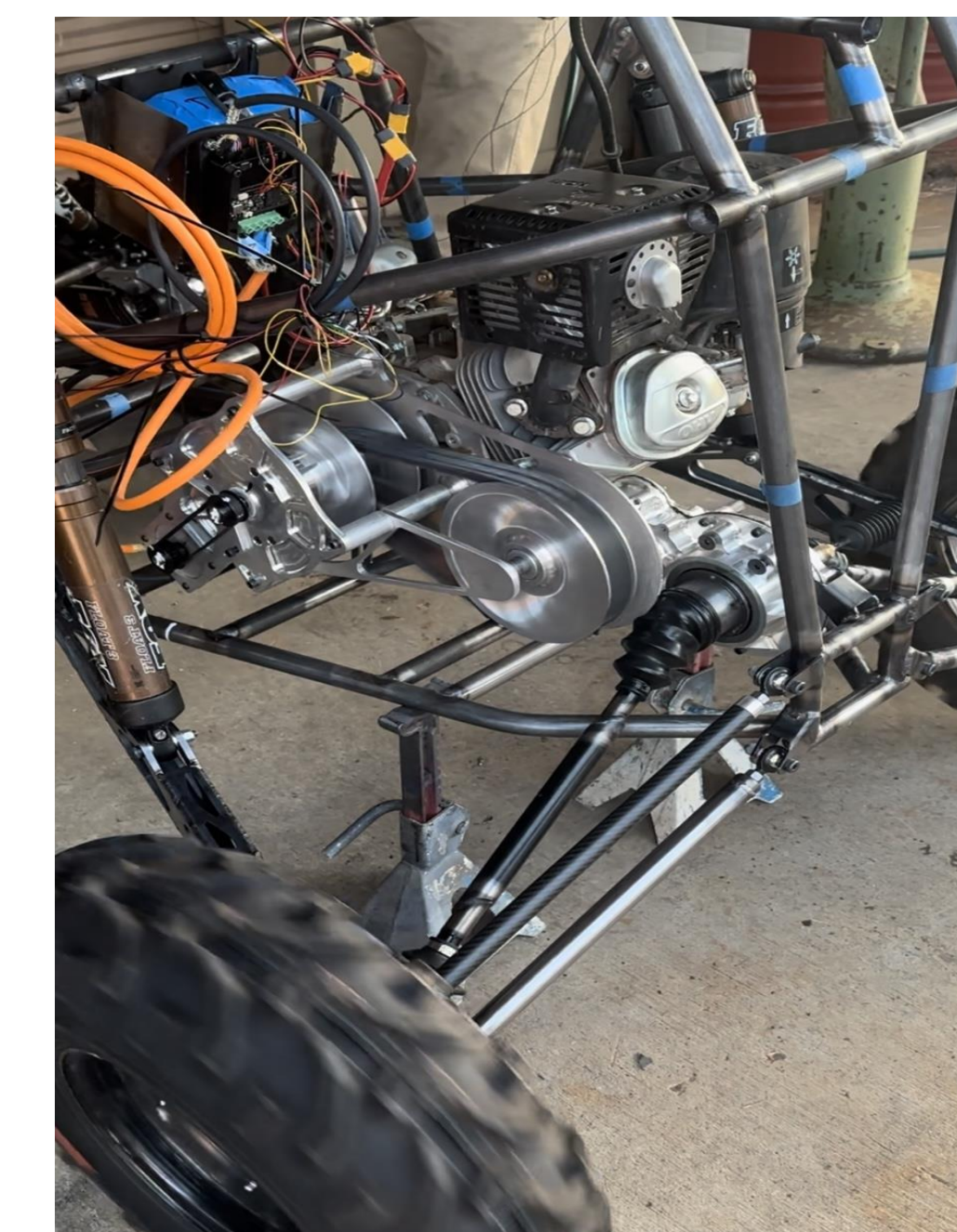
Figure 7: Rear Gearbox / eCVT Assembly
