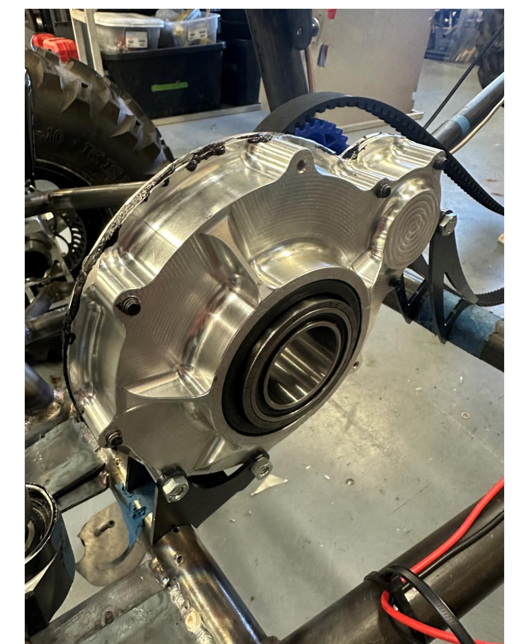
Figure 8: Front Gearbox / 4WD Assembly
