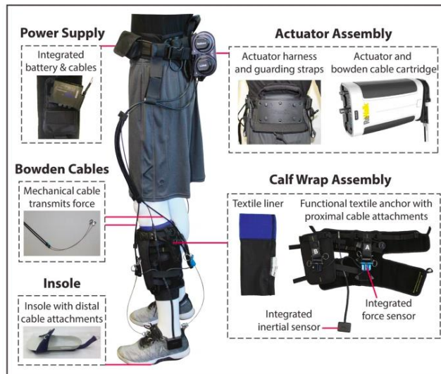
Figure 4: Restore Exosuit by ReWalk
