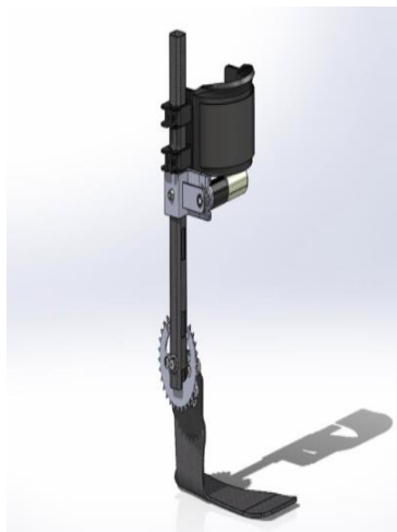
Figure 2: Fully Active Chain and Sprocket Ankle Exoskeleton for Rehabilitation Assistance
