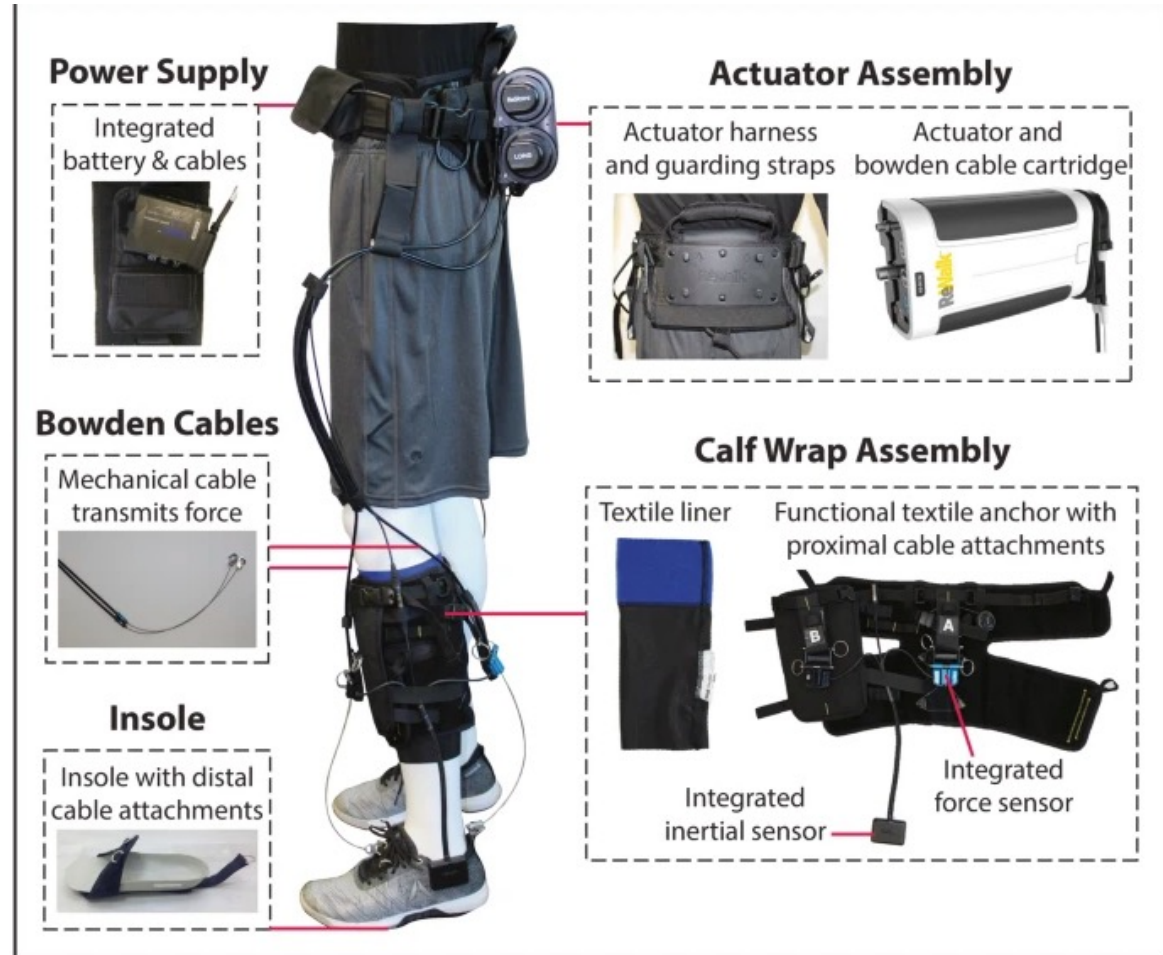
Figure 2: Diagram of the Rewalk Restore Soft Robotic Exosuit
