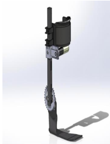
Figure 2: Fully Active Chain and Sprocket Ankle Exoskeleton for Rehabilitation Assistance
