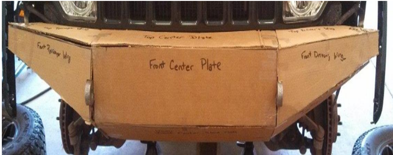
Figure 3: Cardboard Bumper Fitment test comparison
