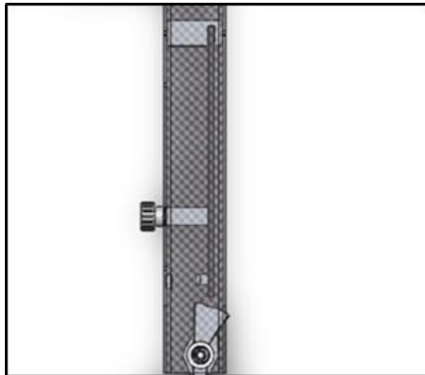
Figure 16: First semester carbon fiber enclosure and leaf spring design
