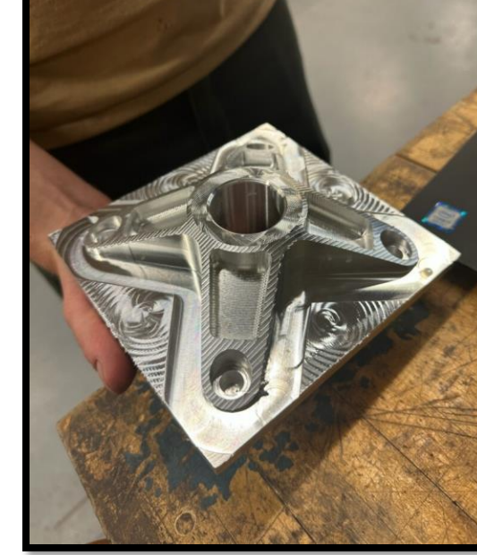
Figure 4: Hub Made Within CNC
