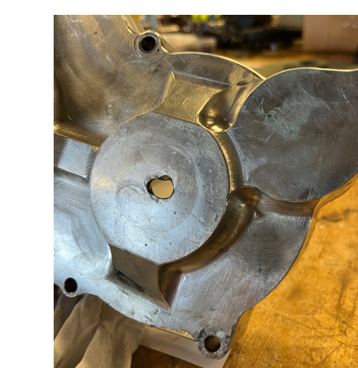
Figure 9: Wear observed on gearbox
