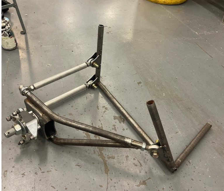
Figure 8 8: Rear Suspension Prototype V2
