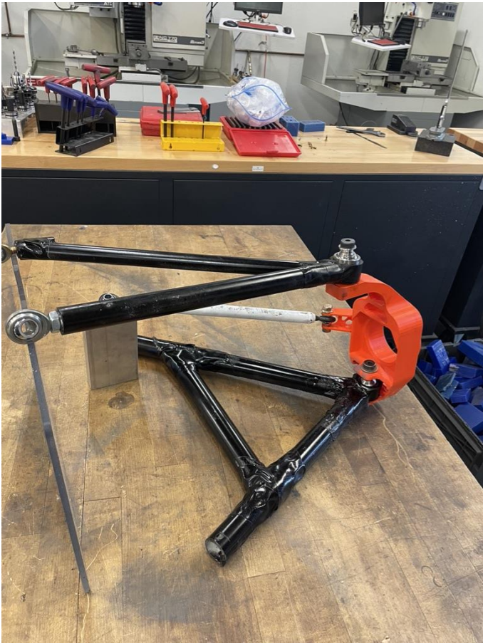
Figure 14 14: Upper and Lower Control Arms
