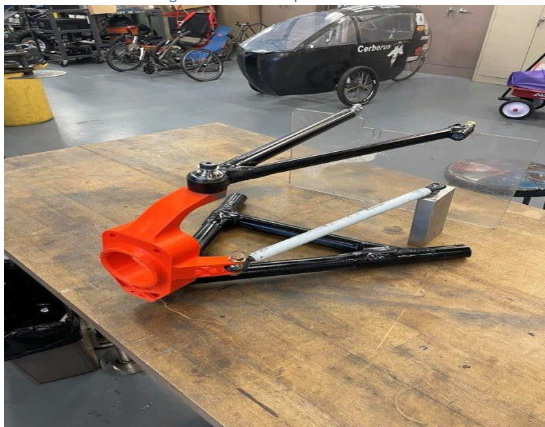
Figure 4 4: Front Suspension Final Prototype
