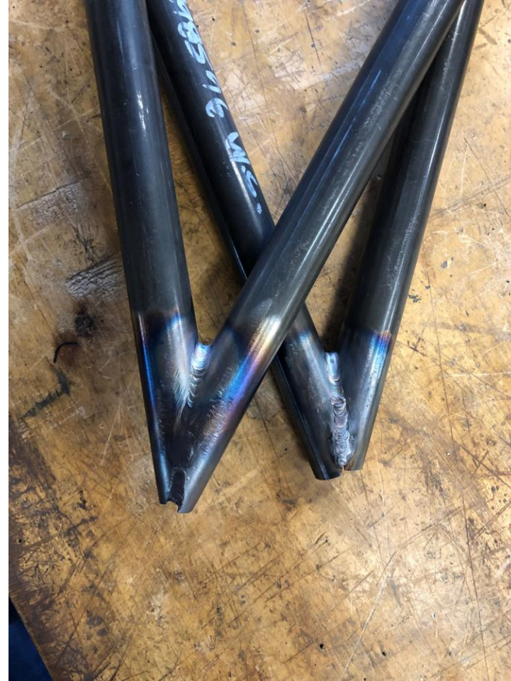
Figure 3: Lower A-Arm Welded
