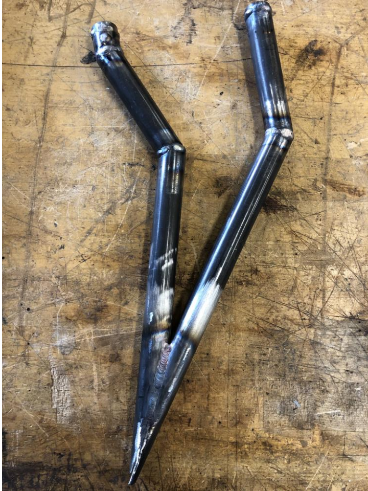
Figure 2: Upper J-Arm Welded
