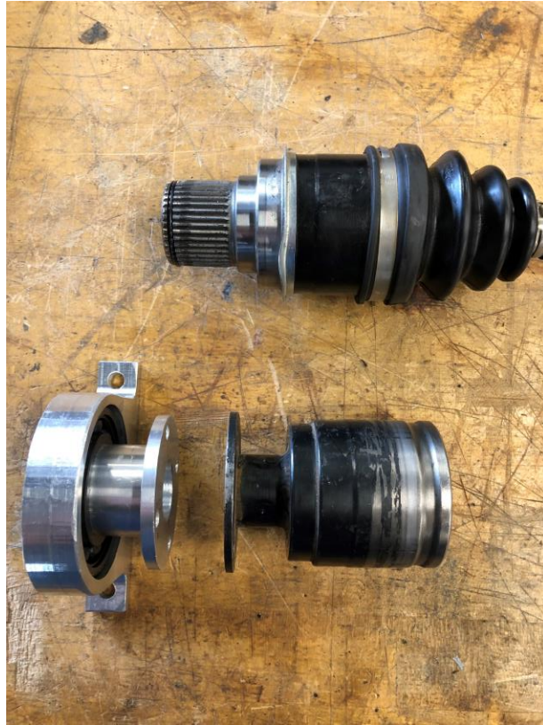
Figure 4: CV Axel Ends Modified for Sprocket Attachment
