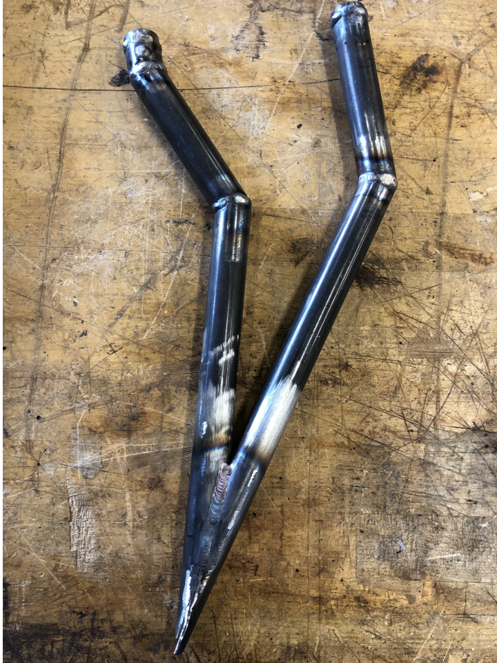
Figure 2: Upper J-Arm Welded
