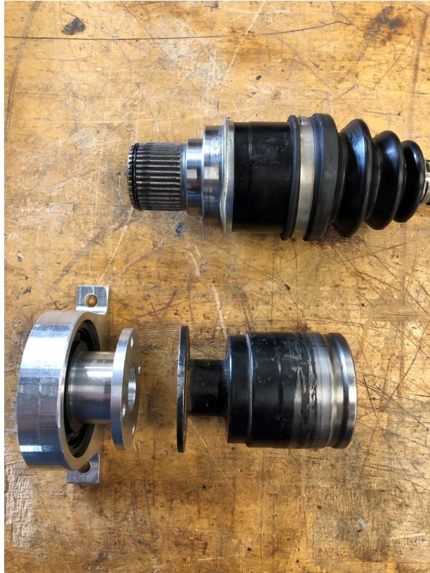
Figure 4: CV Axle Ends Modified for Sprocket Attachment
