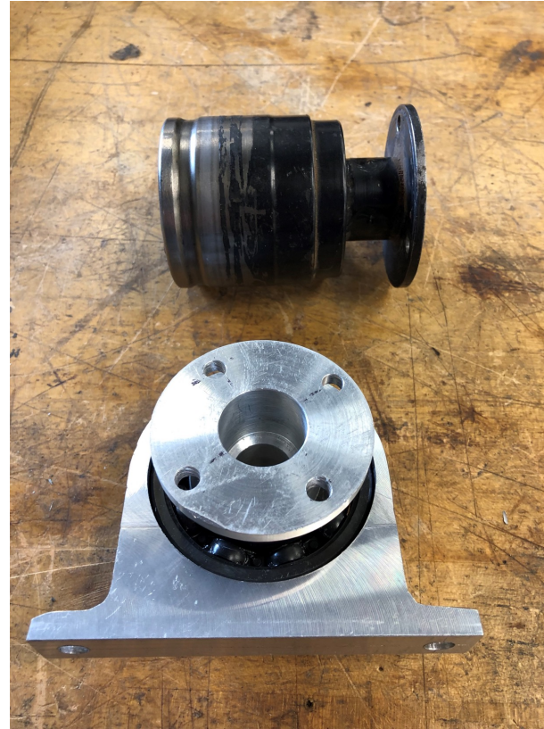
Figure 5: CV Axle Modification with Sprocket Drive Mount
