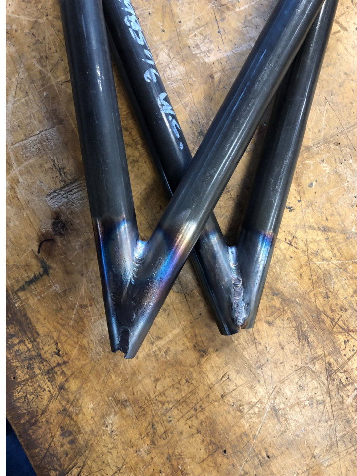
Figure 3: Lower A-Arm Welded
