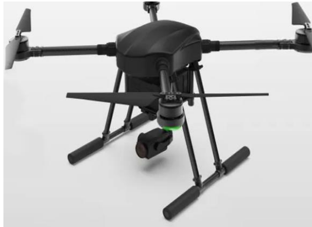
Figure 18: Drone legs attached to the body
