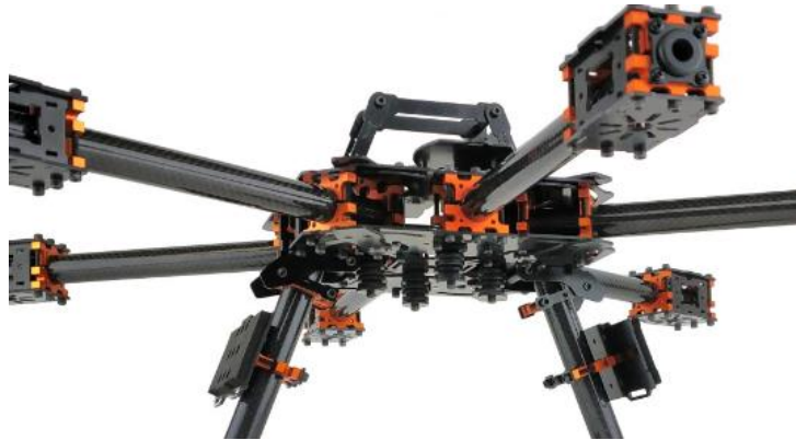
Figure 17: Example of a modular drone frame with swapable components
