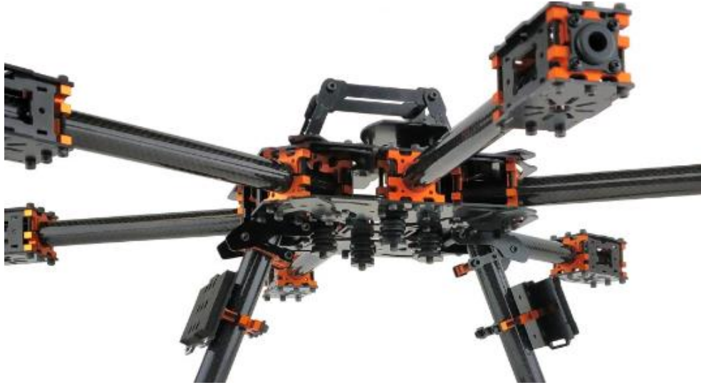
Figure 14: Example of a modular drone frame with modular components
