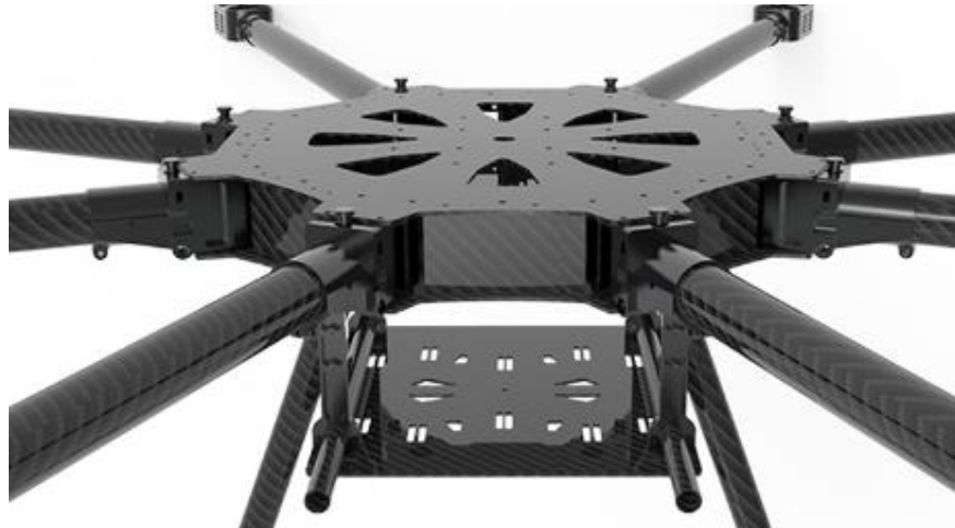
Figure 12: Example of a stacked drone frame
