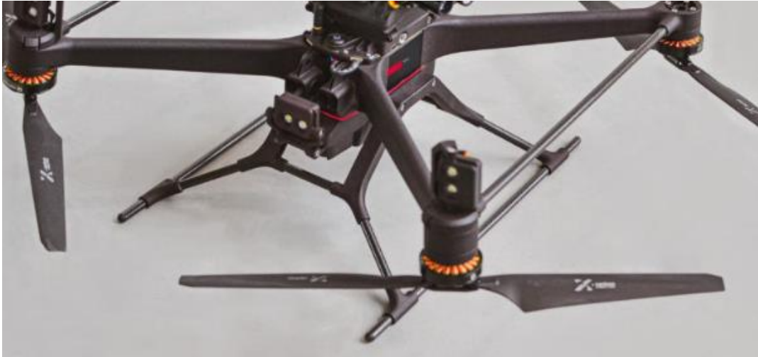
Figure 16: Example of trusses between sets of legs
