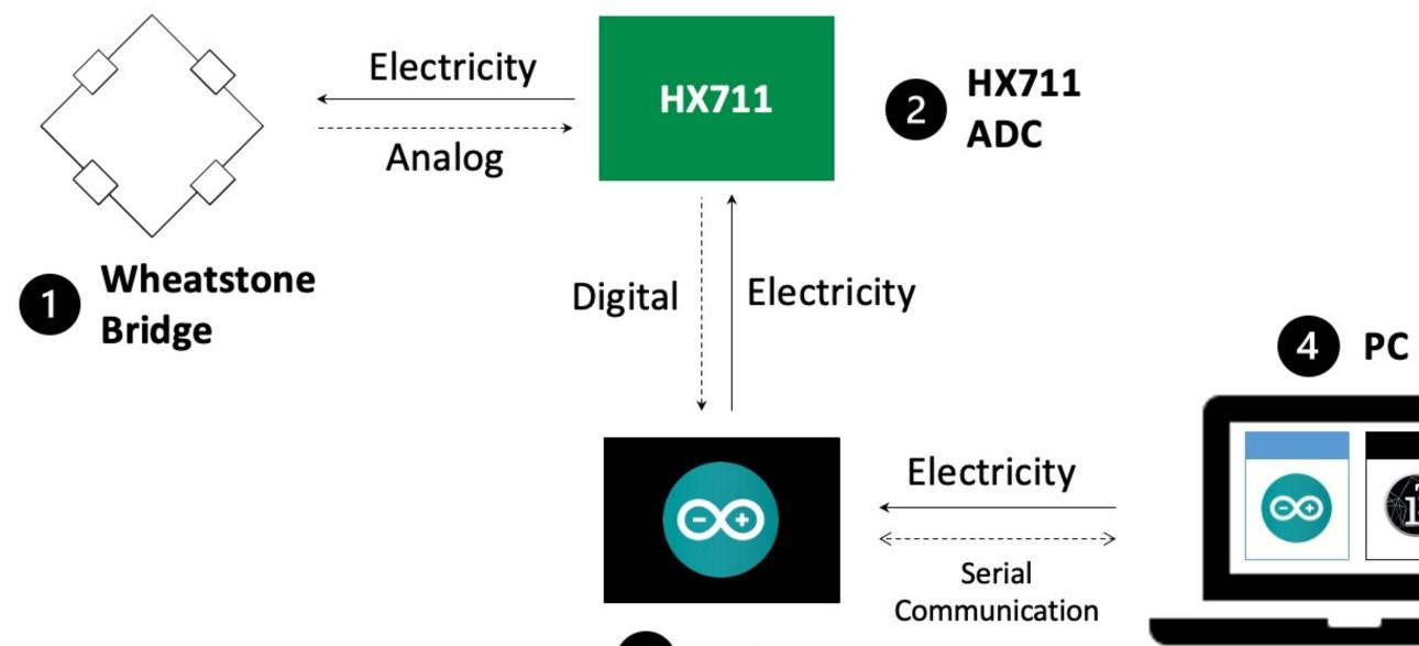
The source of energy of the system is electricity, which is provided by the PC through a USB port. It will be powering the Arduino board, HX711 module, as well as generating a voltage on the Wheatstone bridge circuit to activate the strain gauges. Meanwhile, the signal transfer of the system includes analogdigital conversion on HX711, and serial communication between the Arduino board and the programs installed on the PC.
