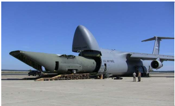
Figure 10: C-5 being loaded with a C-130 fuselage [7]
