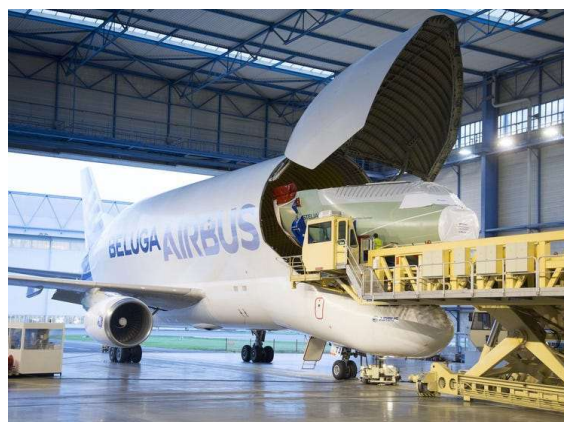
Figure 7: Beluga being loaded with fuselage of another aircraft [7]
