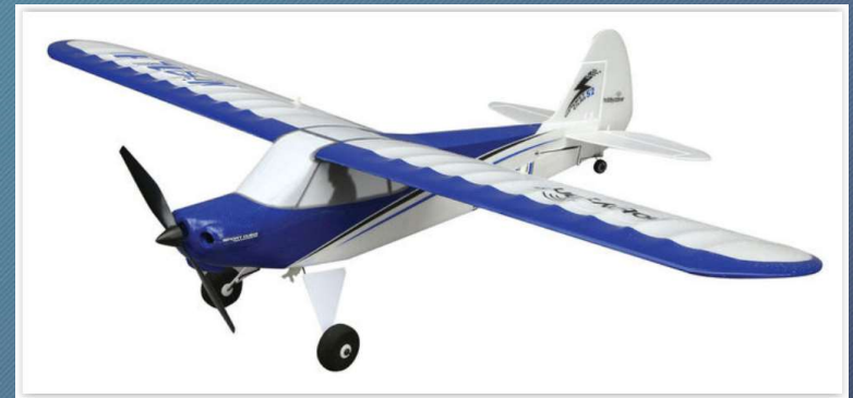
Figure (3): Rc airplane weights less than 0.5 lbs and has a 25-watt motor [3]
