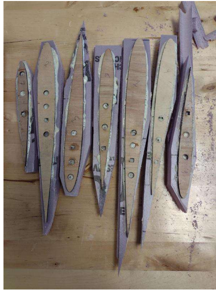
Figure 3: Foam and airfoils cut out prior to glue up
