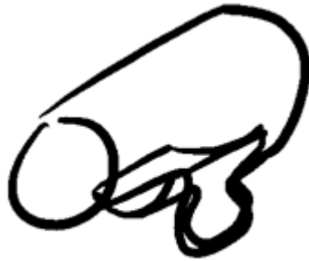
Figure 11: Balloon plug design
