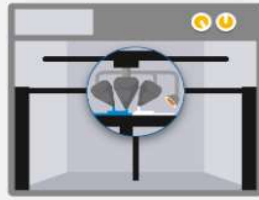
Print heads deposit photopolymer materials and support in ultra-thin layers
