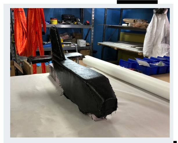
Fuselage Manufacturing Process – Foam Model
